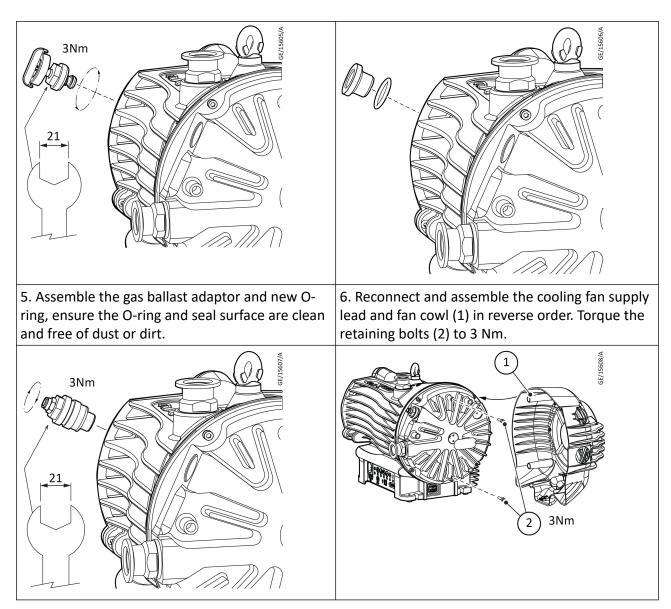
As a precaution, Edwards recommends that a complete a vacuum leak check be performed after this installation.
