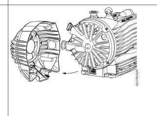
3. Using a 21 mm AF spanner (not supplied), remove the gas ballast control assembly, seat and O-ring.
