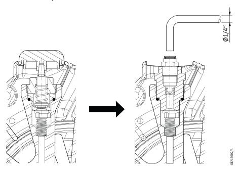
Ensure the pump is switched off before fitting.
